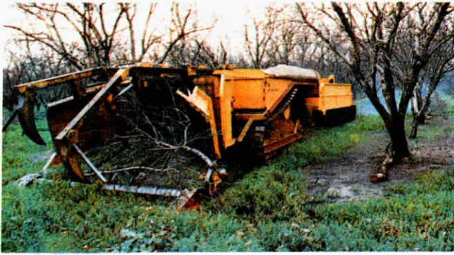
Two huge claws reach out in front to rake trash into the throat of the machine.
