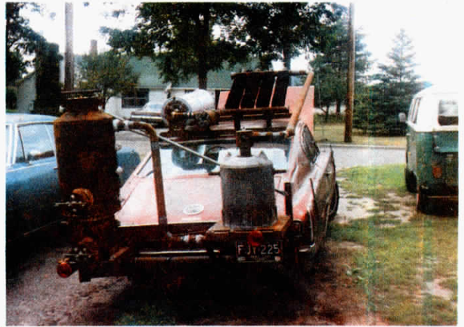
Wood gas from burner, left, goes through a series of scrubbers before it's pulled into the unmodified engine up front.
