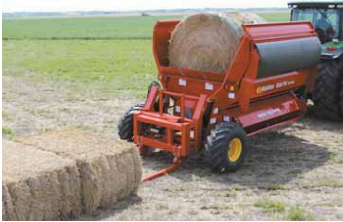
Highline bale processor is equipped with a new twine release system that uses bale's weight to slice twine. Unit lifts bales off the ground for processing.
