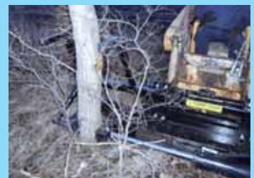
By unbolting cross blade and bolting a push bar/catcher onto boom, operator can shear trees, catch them, and haul them away (above). Boom can also be used to prune tree limbs up to 16 ft. high.
