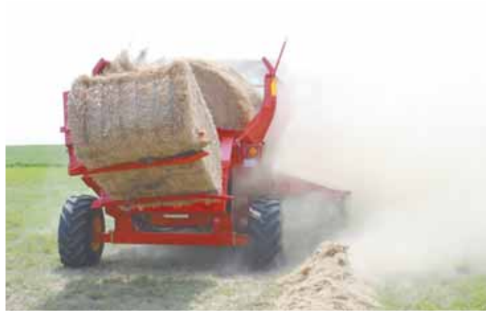
Square bales are turned 180 degrees, putting them in line with machine's flail chopper for optimal processing.
