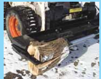
Multi-purpose machine is equipped with a 10-in. tall, 4-way splitter blade with the vertical part welded to boom. Splitter's cross blade is bolted on.
