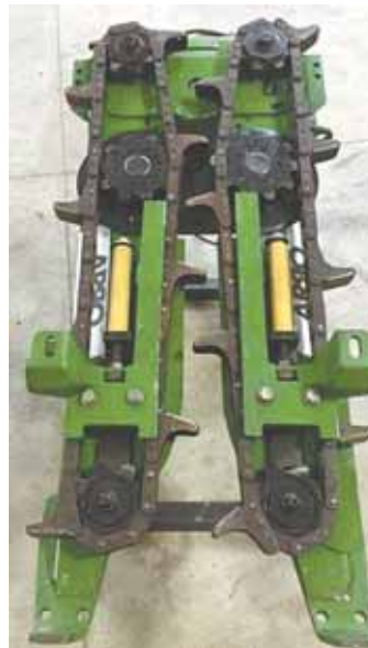
Kopper Kutter kit lets you use a cornhead to harvest crops like sorghum and sunflowers. Kit consists of two 9-in. dia. chain-driven discs with sprockets mounted on back.
