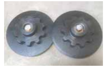
Kopper Kutter kit lets you use a cornhead to harvest crops like sorghum and sunflowers. Kit consists of two 9-in. dia. chain-driven discs with sprockets mounted on back.
