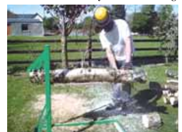
Unit measures 2 ft. wide by 4 ft. tall and weighs about 44 lbs. (above). Teeth quickly release the wood when you're done cutting.
