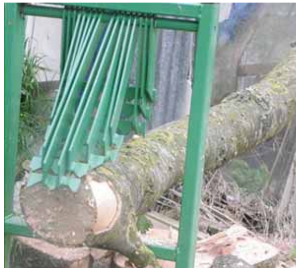
Timbercroc log holder holds logs off the ground while you cut them with a chainsaw. A series of hinged steel teeth with hooks at the end hold log securely in a horizontal position about 2 ft. off the ground.
