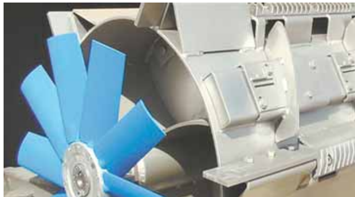
Sunnybrook Welding is testing a new axial fan system to improve crop separation in rotary combines. System pressurizes rotor with a 10-blade fan that forces air into a 3-blade centrifugal fan inside rotor.
