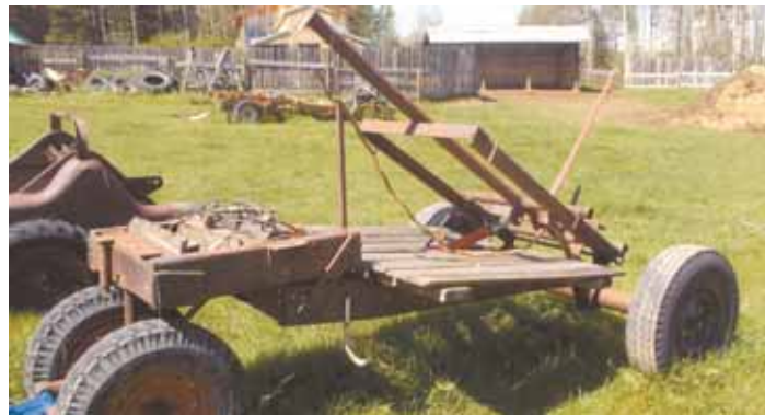
Gary Josephson’s horse-drawn round bale retriever is equipped with an electric-over-hydraulic lift, allowing him to pick up bales and drop them where he wants.
