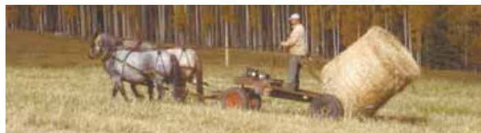
He started with the rear axle and frame off an old trailer and added a front axle with truck wheels under it.
