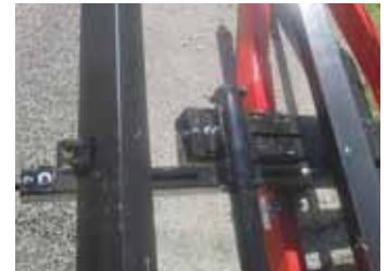
Threaded metal rods run through lengths of slotted tubing that extend across rails. Cradle width, and spacing between cradles, can be adjusted by using an impact wrench to turn rods.
