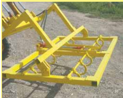
Kornkven also built this bale grapple to handle up to 4 bales at a time. It was featured in FARM SHOW’S Vol. 40, No. 1.
