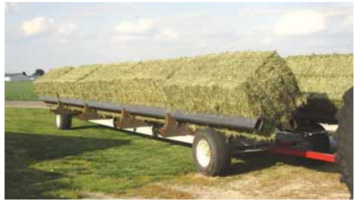
Each cradle consists of 2 adjustable rails made from 4 by 6 rectangular tubing mounted at an angle. Bales can be loaded from either the side or rear.
