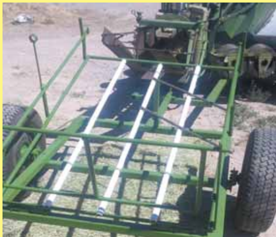
Home-built bale accumulator rides on wheels that go between the furrows on flood-irrigated hay fields.
