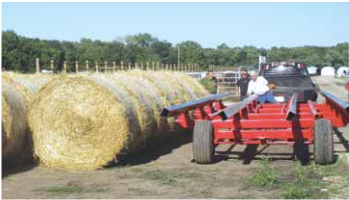
“Lickety-Split” hauler requires no hydraulics or electronics. It’s equipped with two side-by-side, spring-loaded cradles that can haul up to 18 round or 10 big square bales at a time.
