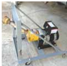
Generator mounts on a rolling frame.
