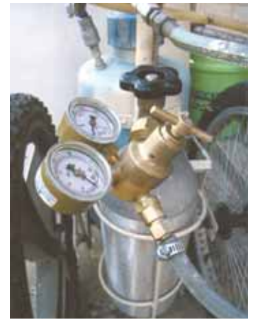
Boehler mounted a 5-lb. carbon dioxide bottle and pressure regulator on a 2-wheeled steel frame, along with the 3-gal. tank and hand wand off a handheld pump sprayer. Carbon dioxide bottle pressurizes tank constantly, eliminating the need to do any hand pumping.
