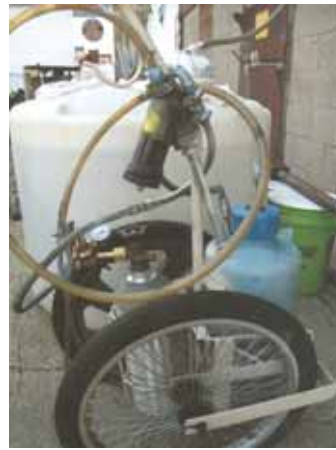
Boehler mounted a 5-lb. carbon dioxide bottle and pressure regulator on a 2-wheeled steel frame, along with the 3-gal. tank and hand wand off a handheld pump sprayer. Carbon dioxide bottle pressurizes tank constantly, eliminating the need to do any hand pumping.
