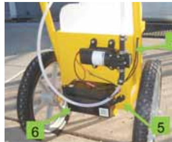
Battery-operated spray cart continuously sprays a variety of liquid products directly from a 5-gal. bucket or 2 1/2-gal. jug. Pump (below) is controlled by a switch on handle.
