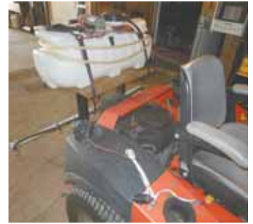
Dan Schultz got tired of using his 4-gal. backpack sprayer so he mounted a 15-gal. spot sprayer on back of his riding mower. “It worked great as a spot sprayer, but then I decided I also wanted a boom,” he says.
