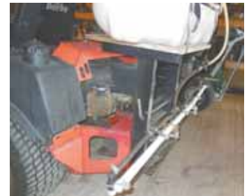
Dan Schultz got tired of using his 4-gal. backpack sprayer so he mounted a 15-gal. spot sprayer on back of his riding mower. “It worked great as a spot sprayer, but then I decided I also wanted a boom,” he says.
