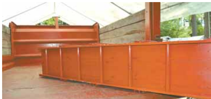
“An aluminum ladder makes a good frame for a big toolbox because it’s strong yet lightweight,” says Bernella.
