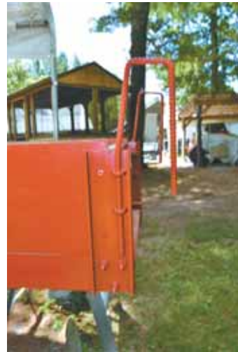
To suspend the box from the sides of the dump bed, he bent a couple sections of rebar that hook over the bed sides.
