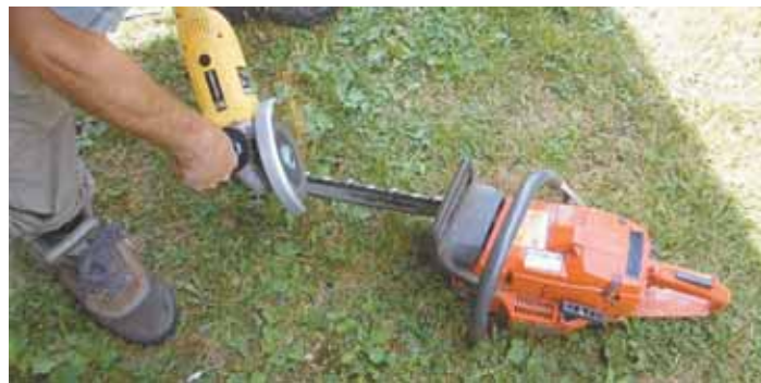
Matthias Wandel uses an angle grinder with a cutoff wheel to quickly sharpen chainsaw chains.
