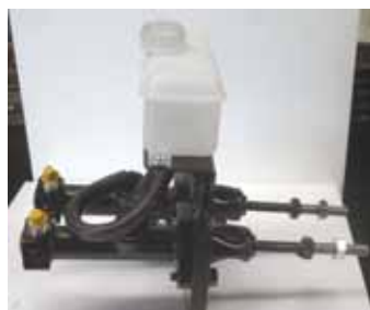
Conversion kit replaces faulty master cylinders on older Deutz tractors.
