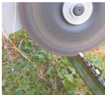
"It's critical to get the right angle and to be careful not to cut the links," he says.
