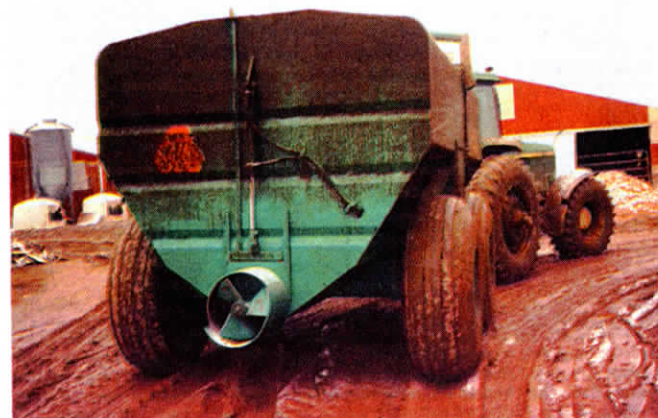
The 18-in. dia. propeller turns in the same direction whether loading or spreading.
