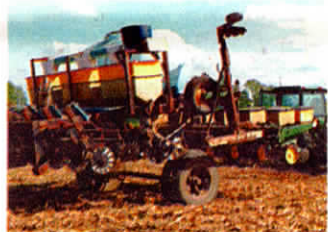
Down pressure on each pair of row cleaners is provided by a 2 1/2-in. dia., 8-in. long air cylinder.
