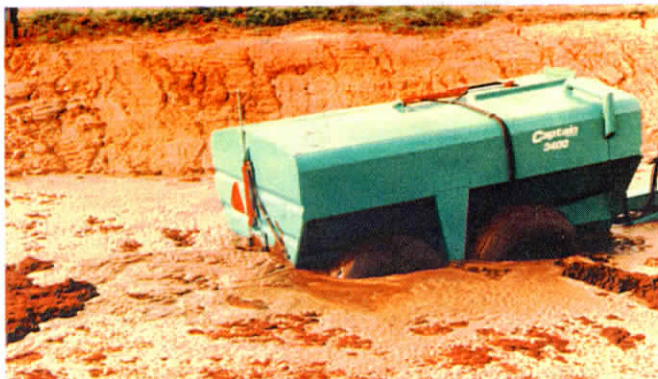
Spreader is backed down into pit until propeller is completely under manure. To load, you open a hydraulically-controlled gate on back and start the propeller.
