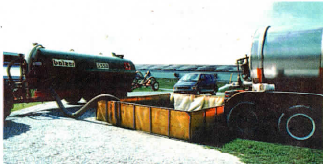
The 3,000-gal. portable canvas holding tank keeps both semi tanker truck and applicator busy with almost no down time.
