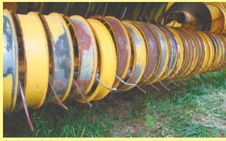
Baler pickup with bent, rusted steel bands.
