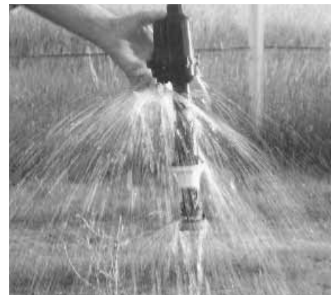
Filter fits between the hose and the regulator on center pivot drop nozzles (left). To flush out sediment you just push up a small release valve on side of filter.
