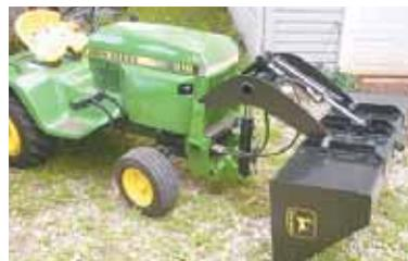
Loader’s boomerang-shaped lift arms are raised or lowered by a single hydraulic cylinder. Another cylinder is used to tilt bucket.
