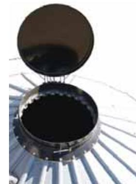
Kit enlarges lid opening on bins by up to 70 percent, making it easier to position big grain augers when filling bins. Kit comes with a new, larger bolt-on collar and a larger cable-controlled, spring-hinged lid.
