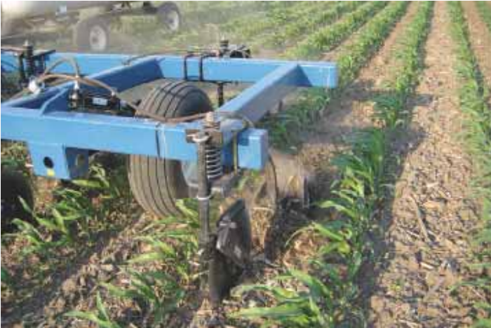
John Miller says his new “sealer shield” lets you apply nitrogen to small corn plants at fast speeds, without covering them up.
