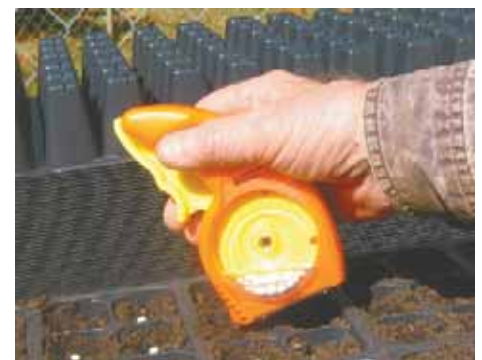
Hand seeder uses a seed disc to singulate seeds just like full-size farm or garden planters.
