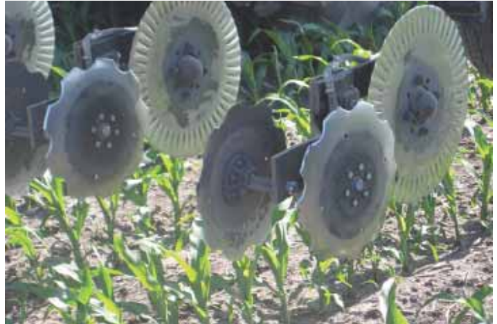
As applicator is pulled through field, pairs of offset coulters gather soil disturbed by the knife and redirect it to cover the nitrogen so it won't be lost.
