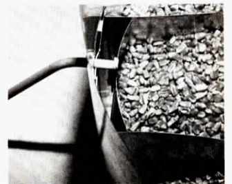
When bin is empty, left, handle points straight down. At right, grain pushes paddle against bin side, lifting the handle to signal the bin is full.
