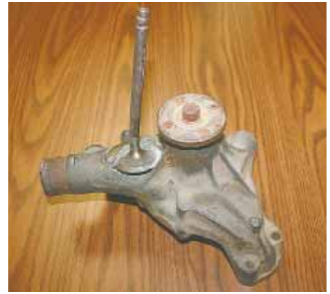
Magna 777 rod provides machinable welds that won't crack on most types of cast iron. Photo shows a steel valve welded to a cast iron pump.
