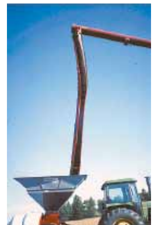
The 30-ft. flexible spout extension makes it easier to fill grain bagger with an auger and semi truck, instead of having to use a smaller grain cart or tandem axle truck.
