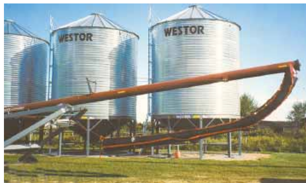
The 30-ft. flexible spout extension makes it easier to fill grain bagger with an auger and semi truck, instead of having to use a smaller grain cart or tandem axle truck.
