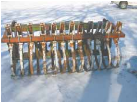
Harlen Grovom built this 7-ft. wide grapple fork out of cultivator and chisel plow shanks.
