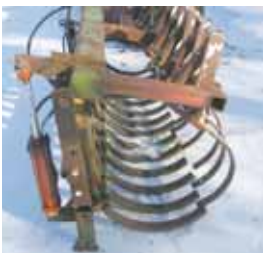
He used 4 by 2 tubing off an old cultivator to build the frame, which supports 2 rows of spring-loaded shanks spaced about 7 in. apart.
