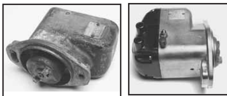
These photos show Calin magnetos before and after they're rebuilt.
