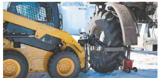
Tire Jogger uses hydraulic cylinders to grab, hold, and rotate large tires from the safety of a skid loader. Two large metal "arms" securely grip and hold the tire.
