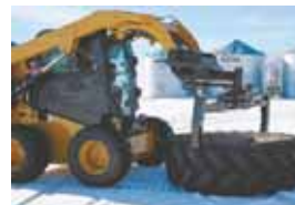
Tire Jogger uses hydraulic cylinders to grab, hold, and rotate large tires from the safety of a skid loader. Two large metal "arms" securely grip and hold the tire.
