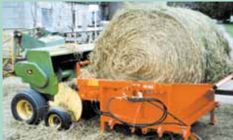
Machine unwinds bale directly over pickup reel of any small square baler. Here, a 5-ft. wide, 6-ft. dia. bale weighing about 1,200 lbs. is being unwound into a Deere 336.
