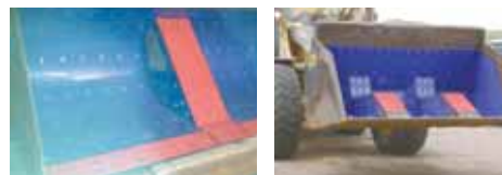
Dave Julian came up with a way to line loader buckets with UHMW poly. "Nothing sticks to it," he says. He cuts poly to fit, then shapes and bonds it to the bucket with metal fasteners.
