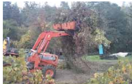
Bernier attaches chain and a pair of 70-lb. tractor suitcase weights to his loader bucket to hold big loads in place.
