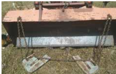
Bernier attaches chain and a pair of 70-lb. tractor suitcase weights to his loader bucket to hold big loads in place.
