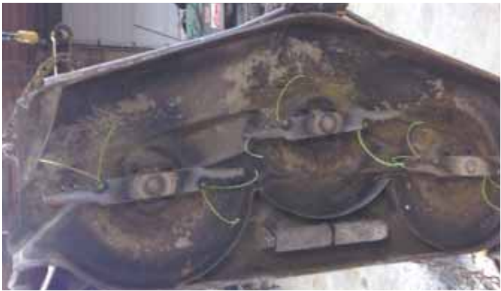
Pairs of 18-in. long weed trimmer lines loop through holes that Steven Simpson drilled into the mulching blades on his Deere riding mower.
