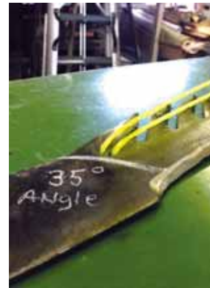
Simpson drilled the line mounting holes at about a 35 degree angle to the blade, which keeps the lines spaced about 1/4 in. apart.
