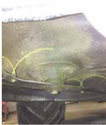
Simpson drilled the line mounting holes at about a 35 degree angle to the blade, which keeps the lines spaced about 1/4 in. apart.
