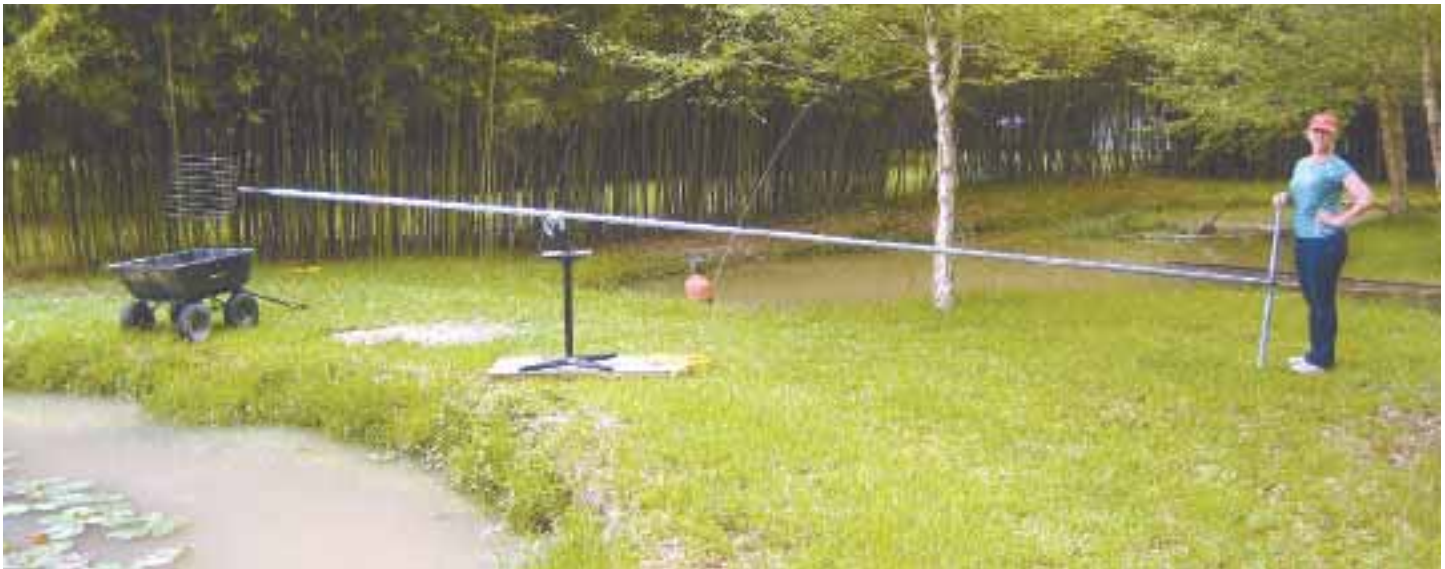
Jody Taylor uses a long, swivel-type “muck scoop” to dig fertile muck out of ponds and dump it into a wheelbarrow, which he then hauls to his garden.
