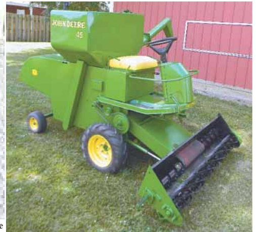
Combine’s 5-ft. header is fitted with three 21-in. reel mowers mounted side-by-side.
