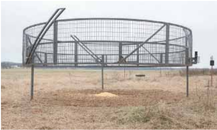
Drop trap is shown here ready to trigger, as seen from a computer monitor or cell phone.
