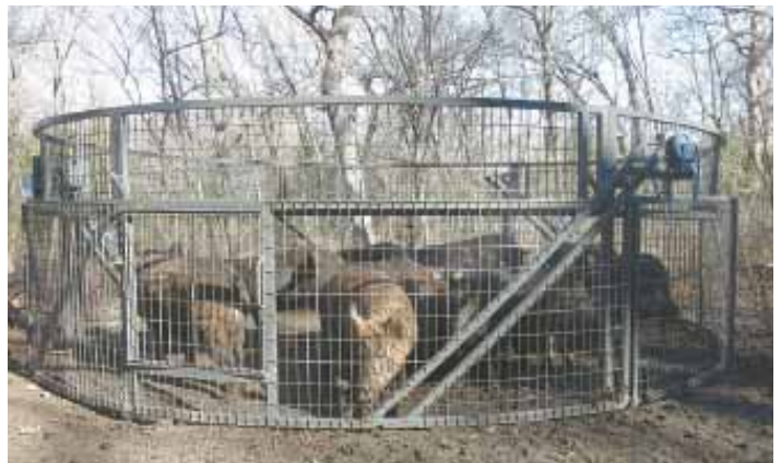
When the operator triggers the corral via cell phone or remote control, the outside ring falls to the ground.
