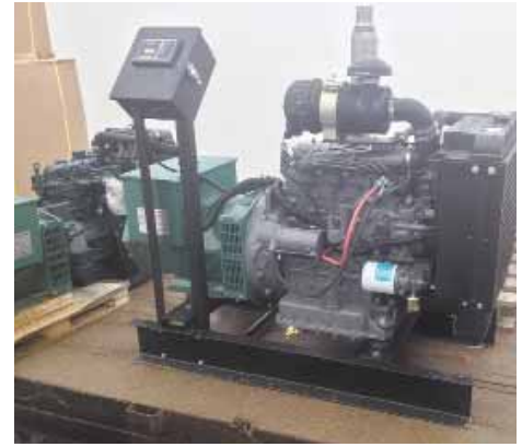
“Reefer” engines can be used to make low-cost gensets, says Joas Bontrager, who offers low hour Kubota engines with new generators.
