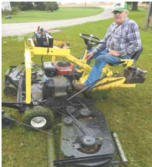
Starting with an old 3-wheeled bean buggy, Virgil Davis built this riding mower that cuts a 10-ft. wide swath with three 42-in. mower decks.
