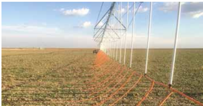
Dragon-Line system drags specially-designed flexible hose and emitter tubing behind a center pivot irrigator, and releases water directly onto the soil surface.
