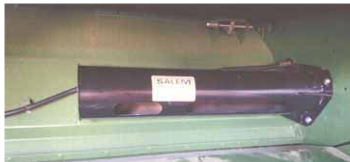
Bolt-on "tailboard trash blower" for Deere combines directs air onto tailboard to keep it free of trash, dirt and dust.
