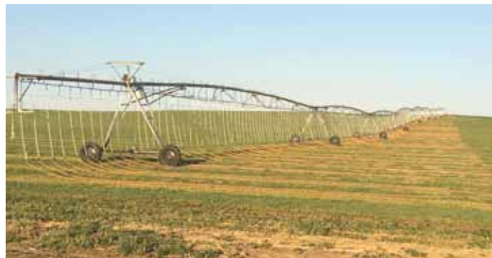
Tubing attaches to the end of a rigid or flexible drop and/or a manifold. System can result in 20 to 50 percent water savings, says the company.
