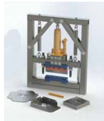
Compact benchtop press brake makes use of a common 20-ton bottle jack. A backstop allows material to be bent in the same location every time.
