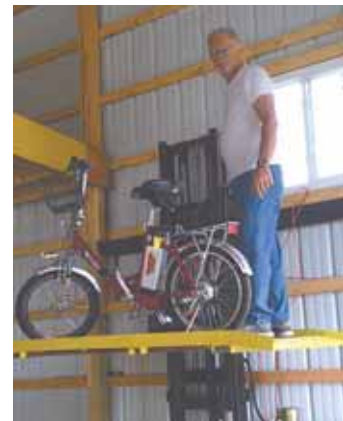
Larry Wood converted an old forklift mast into a shop elevator by building a platform onto the mast in place of the forks. Elevator is controlled by electrically-powered hydraulics.
