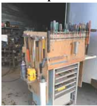
An anesthesia cart was converted into this portable tool cart.
