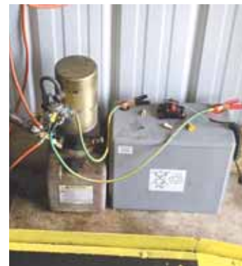
Larry Wood converted an old forklift mast into a shop elevator by building a platform onto the mast in place of the forks. Elevator is controlled by electrically-powered hydraulics.
