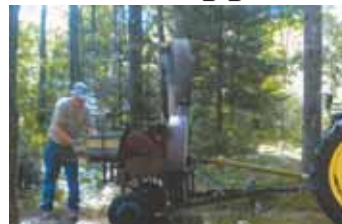
Jones uses his Deere "B" 25 hp tractor to operate the wood chipper.
