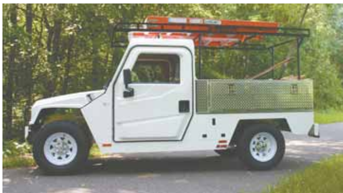
Off-road EXV-2 E-truck only costs 2 cents per mile to charge and requires limited maintenance, thanks to its lithiumion batteries and electric drive.
