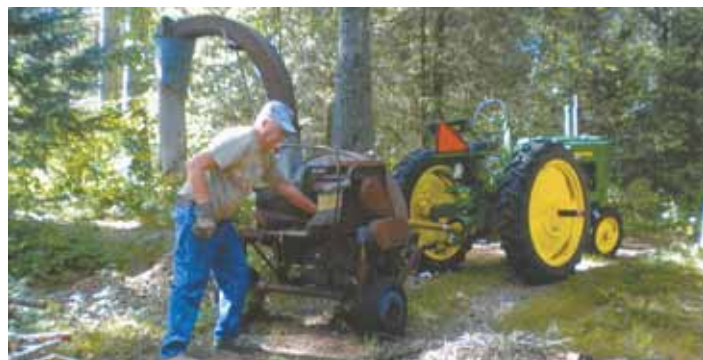
"It works great," says Vance Jones, who converted an old Case flat belt-driven silo filler into this heavy-duty wood chipper.
