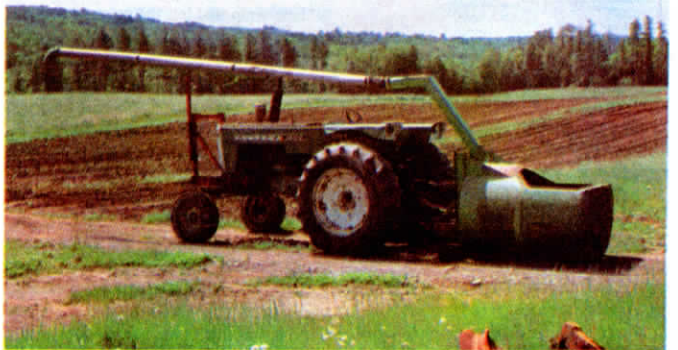
Receiver is fitted with 1,000-rpm pto-driven pump that discharges through 6-in. fill pipe that runs up and over top of tractor.
