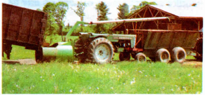
Manure is unloaded from truck into receiver, then pumped into spreader.
