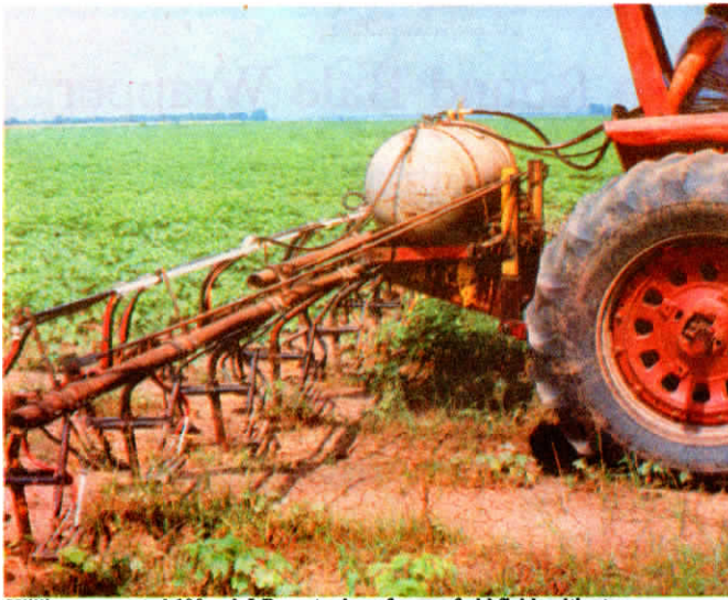
Williams mounted 100-gal. LP gas tank on frame of old field cultivator.
