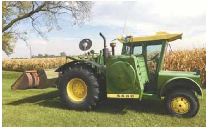
He cut the combine's frame apart and moved the steering wheels from the back to the front. The hood was made from the back section of the combine.
