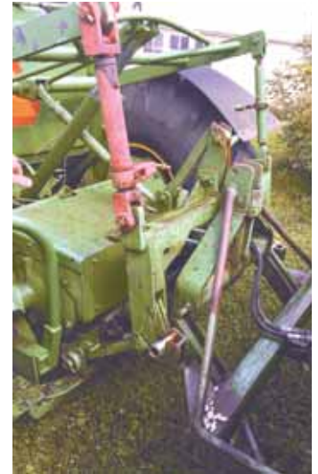
Back end of machine is fitted with a 3-pt. hitch, pto, and live hydraulics.
