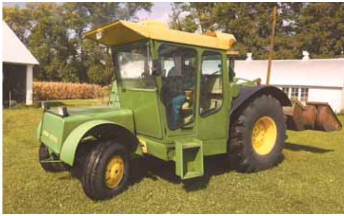
"When I retired my Deere 6600 combine after nearly 30 years of service, I hated to send it off to the junk yard. So I converted it into a lo-boy tractor," says Virgil Davis.
