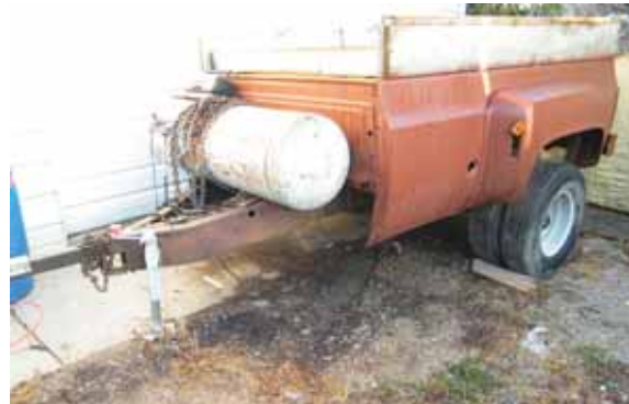
Gary Swensen converted a 1-ton, 4-WD dual-wheeled pickup into this handy field trailer. A converted 80-gal. propane tank on front provides an inexpensive portable air supply.
