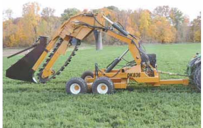
Denny Kirian builds 3 models of rugged DK Trenchers in his Ohio shop. This new pull-type model is mounted on a tandem-wheeled cart with walking beam axles.
