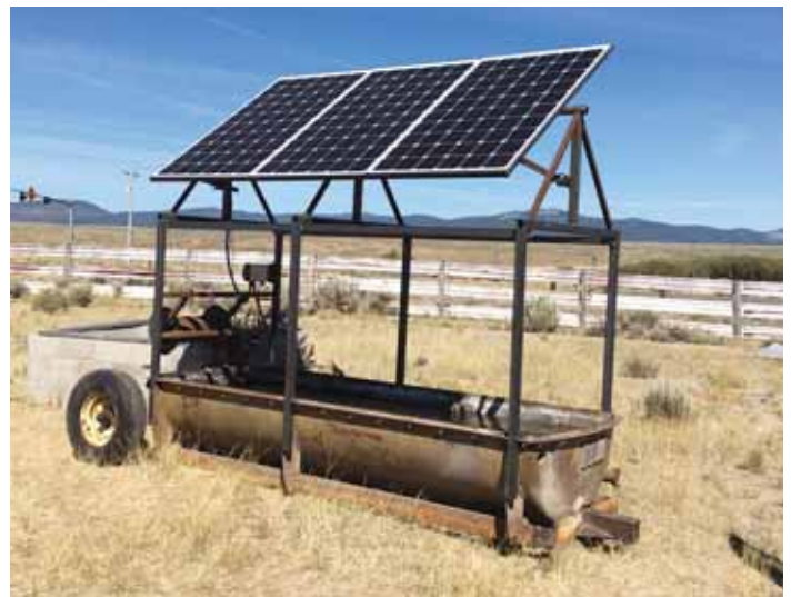
"It has a lot of capacity and can be towed at highway speeds," says Jack Vernon about the portable solar watering system he built. He uses it on ranchland pastures scattered miles apart.
