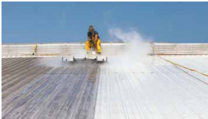
Les Schmidt built this steam washer to clean metal roofs on dairy barns. Washer's 4-ft. wide deck has 4 high-pressure nozzles underneath that spray 160-degree water.
