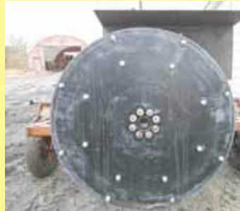
Metal fender over flywheel helps keep dirt from flying up onto tractor.
