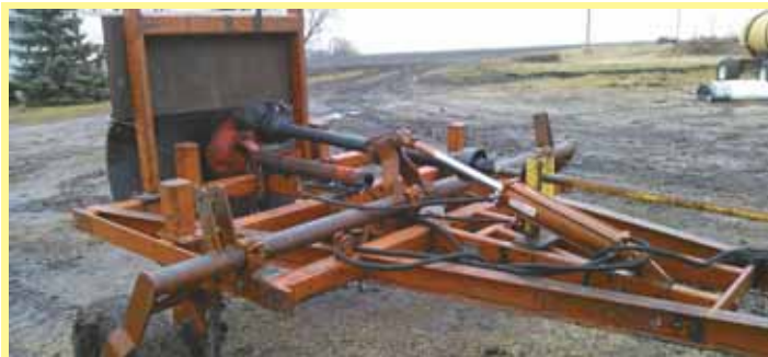
Leroy Groening built this rotary ditcher to dig drainage ditches on his Manitoba farm. He made the ditcher from a cultivator frame fitted with a combine drive axle that pto-drives the flywheel.
