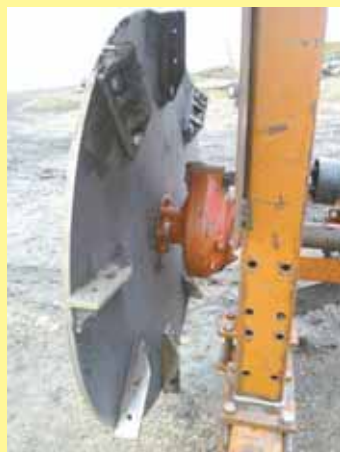
Ditcher’s 59 1/2-in. dia. flywheel is made from 3/4-in. thick steel plate and has 8 paddles bolted onto it.
