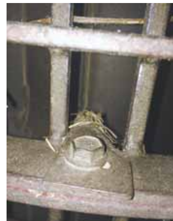
Instead of buying a residue chopper for his older combine, Brent Huneycutt bolted sections of sickle blades to the grates.
