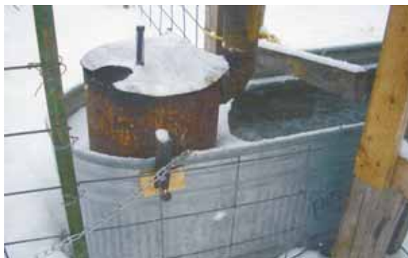
To keep water from freezing in his stock tank, Sam Pajari used a 100-gal. propane tank to make this wood-fired heater.
