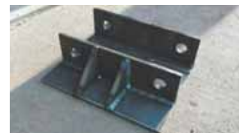
Four ripper shanks spaced 16 in. apart are bolted on back of I-beam which bolts onto backhoe arm with a pair of homemade steel brackets.
