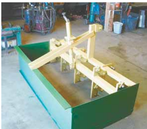
Pat Burrington built this 6-ft. wide, 3-pt. mounted "quick-adjust" box scraper. A 4,000-lb. trailer screw jack is used to raise and lower scraper's ripper teeth.
