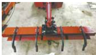
Four ripper shanks spaced 16 in. apart are bolted on back of I-beam which bolts onto backhoe arm with a pair of homemade steel brackets.
