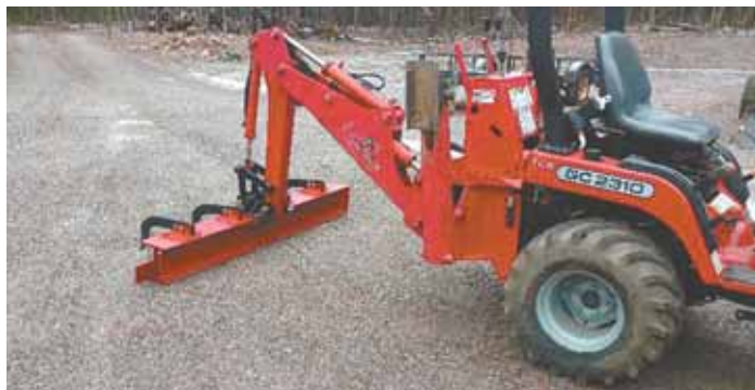
Backhoe-mounted driveway grader was built out of a 5-ft. long square I-beam. It can be tilted forward to use it as a blade, and backward to dig up to 8 in. deep.
