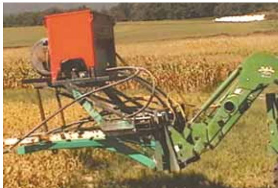
Virgil Gutshall and his son mounted this Gandy air seeder on their front-end loader. “We use it to seed cover crops in soybeans before combining. It gives the crop more time to grow before winter sets in,” says Virgil.
