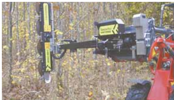
Loader-mounted Quadsaw uses 4 high-speed rotating blades to cut cleanly through tree branches and shrubs.
