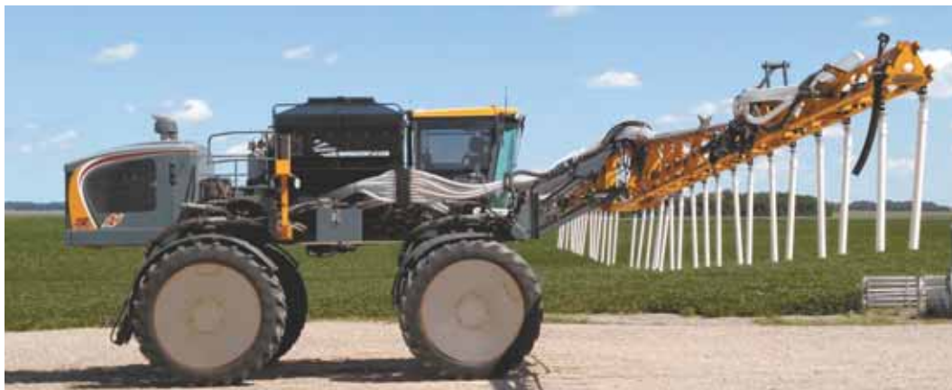
Bryan Biegler fitted this 80-ft. high clearance sprayer with a Gandy air seeder and a series of pipes that hang from the sprayer boom. He says it works great to plant cover crops in late season corn.
