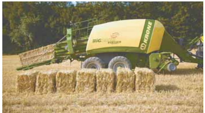
Krone's "BiG Pack" 870 baler produces a single bale about 9 ft. long that contains up to 9 small, individually-tied bales that are easy to handle when feeding.
