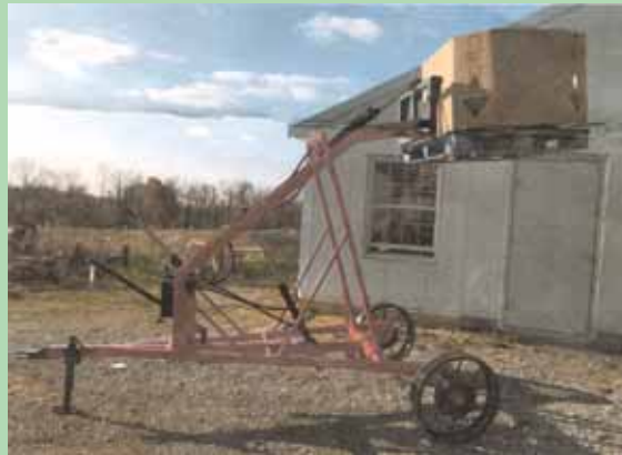
Hoover made a set of pallet forks for the hay mover that can be used to load bins of produce and other material.
