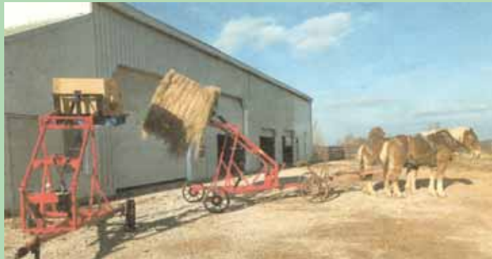
Mark Hoover's horse-powered hay mover uses hand-pumped hydraulic cylinders that can quickly lift big bales into bale feeders or onto trailers.
