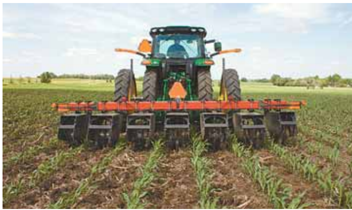
Reservoir Tillage unit runs between rows with 10-in. teeth that fracture soil profile.
