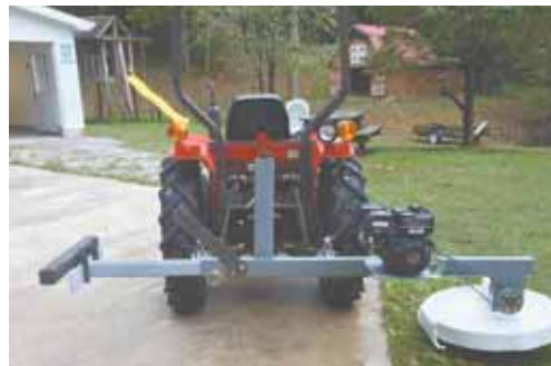
Bill Medley converted an old walk-behind brush cut mower into a 3-pt. model. Mower blade and a new drive motor mounts at one end of arm, with a counterweight at the other end.
