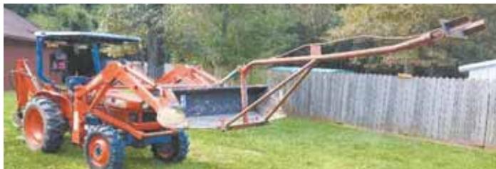
“I built it to lift and push invasive dead trees away from a fence in our pasture, but it’ll lift just about anything,” says Terry Benoit, who converted a 3-pt. mounted boom pole to a loader bucket-mounted unit.
