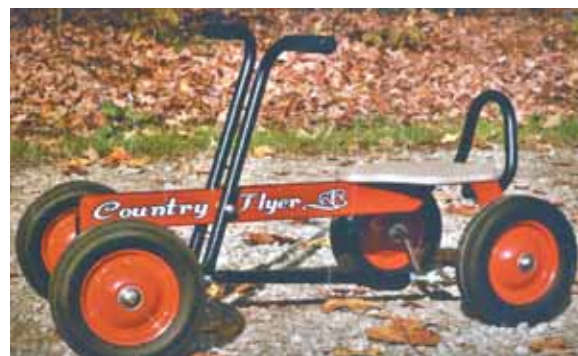
It takes a little coordination to get this go-cart moving, because you have to pump with your hands while using your feet to steer.
