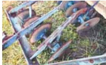
Wickey unbolted 5-in. long axle housing sections from disk and replaced the wooden bearings in them with ones he made from 2 different sizes of pvc pipe.
