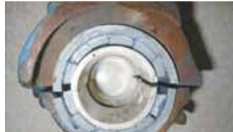
Sections are spaced 1/2 in. apart inside axle housing, to make room for the axle's metal ribs.
