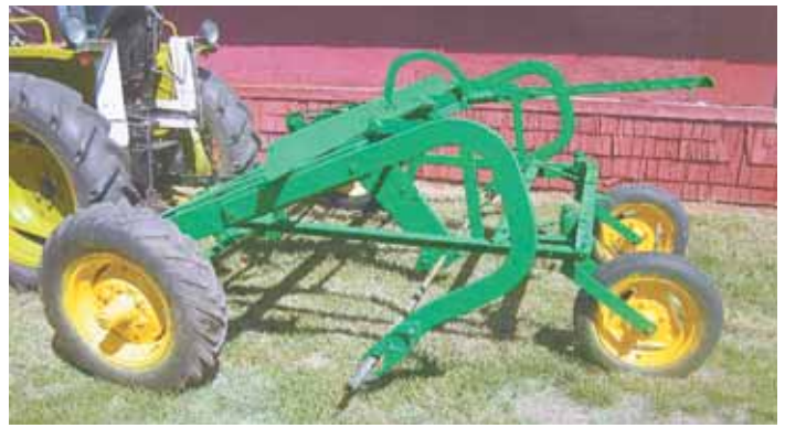
"Weeds really don't like this machine," says Darry Markle, who converted an old 10-ft. wide, Deere pull-type rod weeder to this 8-ft. wide, 2-pt. model.
