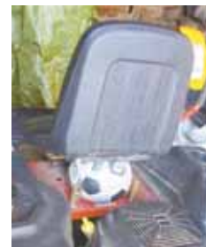
Partially deflated soccer ball fits under tractor seat to smooth out the ride.
