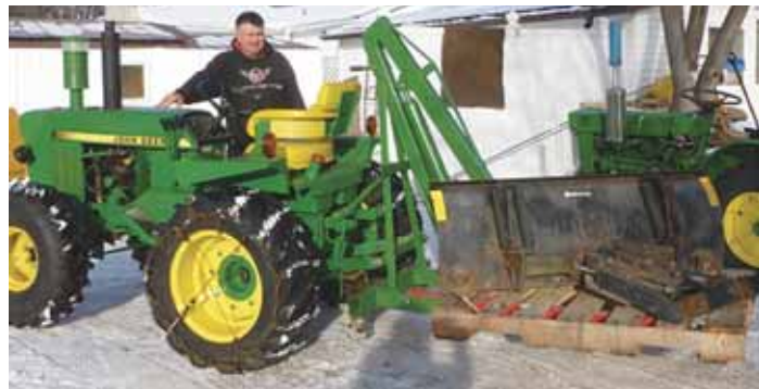
Don Campbell converted a floor shop crane to this 3-pt. mounted crane equipped with forks. Works great to move light loads on pallets and for other jobs.
