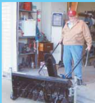
Dale Larsen bolted swivel-type boat trailer jacks to each side of his snowblower. "Makes it much easier to move the blower around," he says.
