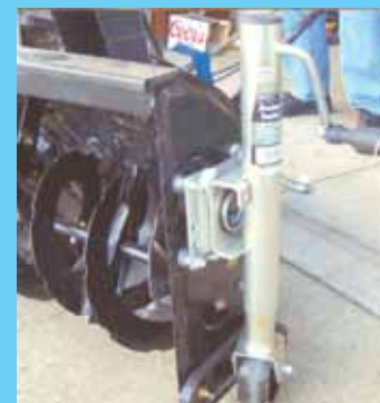
Dale Larsen bolted swivel-type boat trailer jacks to each side of his snowblower. "Makes it much easier to move the blower around," he says.
