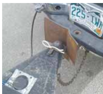
V-shaped steel plate is welded to the receiver hitch behind the ball.
