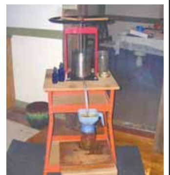
Brian Huckins custom-builds presses that squeeze fluid from herbs infused with alcohol.
