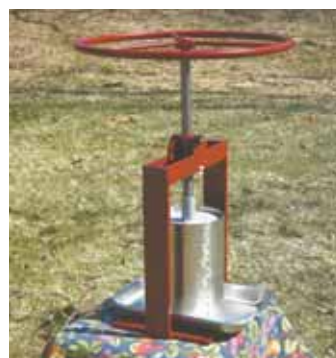
Brian Huckins custom-builds presses that squeeze fluid from herbs infused with alcohol.
