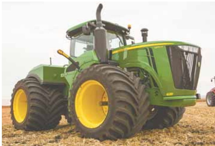
Goodyear's Titan super wide tires are designed for high horsepower, 4-WD tractors. Better traction, less compaction, easier turning and a super smooth ride are promised.
