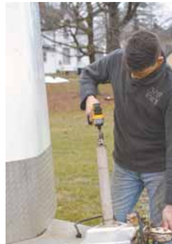
ImpactApp lets you use an impact wrench and socket to crank almost any top-wind jack. It bolts onto jack's shaft.
