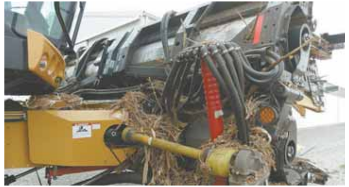
Seed is delivered through a large hose to a manifold behind header, which distributes it through small hoses under each snout.
