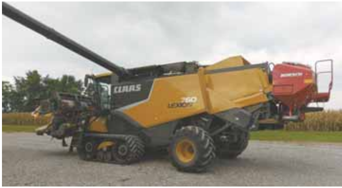
Last fall Drago Indiana mounted a Horsch 80-bu. seeder behind this Claas combine. Seeder's air delivery system spreads cover crop seeds under combine's 12-row header.
