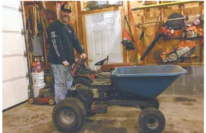
Robert Gunter converted an old Scotts riding mower into this powered wheelbarrow. "It does well in mud and even works good on slopes," he says.
