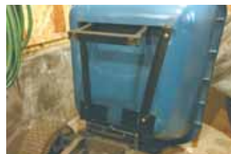
Gunter bolted the plastic tub from an old wheelbarrow to metal brackets on front of mower frame, adding a hinge. Photo at right shows mower before conversion.
