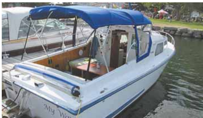
Brian Edmond removed the engine, transmission and fuel tank from his 22-ft. cabin cruiser and converted it to run on batteries and DC motors.
