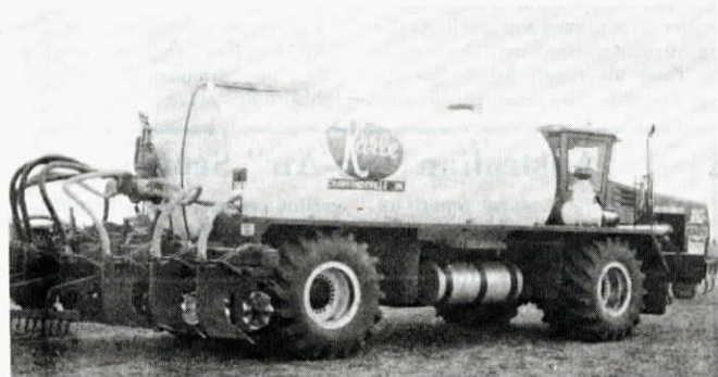
Spreader features huge, spring-loaded injection knives and 6-ft. tall tires.
