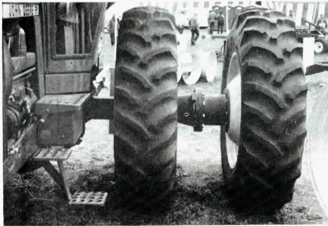
These cast iron hub extensions are one of three types of wheel spacers developed by Unverferth.
